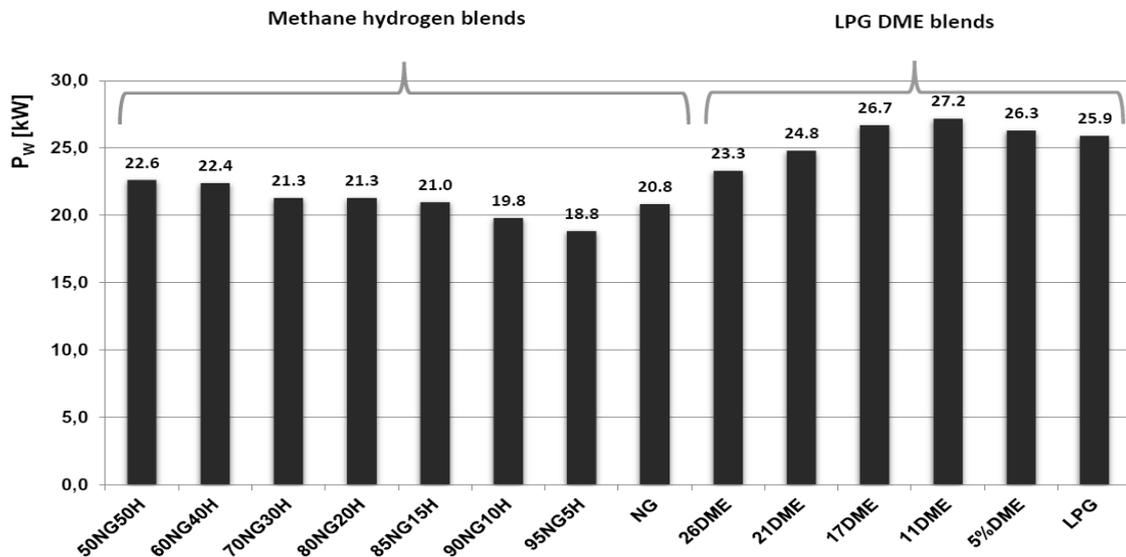
Fig. 3. The variation of power in the wheels, for rpm=2500, 100% load,  $\lambda=1.0$
