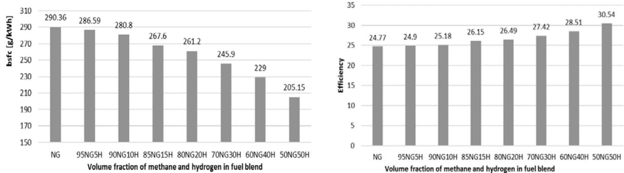
Fig. 9. Brake-specific fuel consumption and engine efficiency for all methane and hydrogen mixtures
