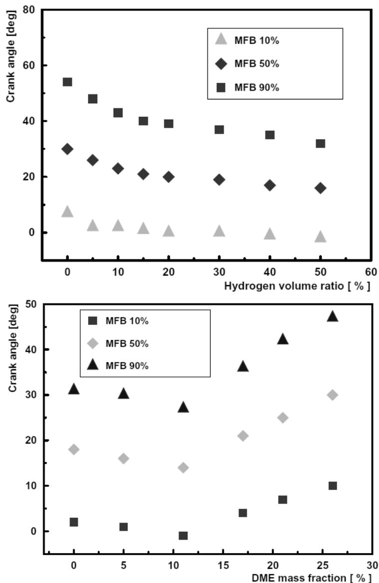
Fig. 8. Variations of CA corresponding to 10, 50, and 90% MFB for various cases of hydrogen share and DME mass fraction; 2500 rpm, load 100%, spark advance 30°,  $\lambda = 1.0$
