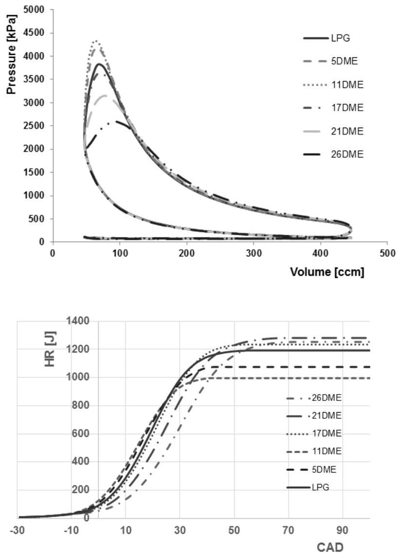
Fig. 6. p–V diagram and heat-release function for the engine fueled by LPG–DME mixtures, at 2500 rpm; WOT and  $\lambda = 1.0$
