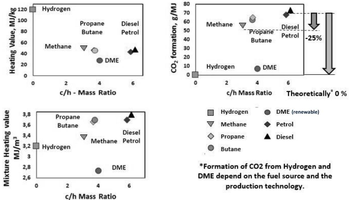
Fig. 1. Main properties of selected gaseous fuels as a function of c/h ratio (at p=100 kPa, T=283 K, λ=1)
