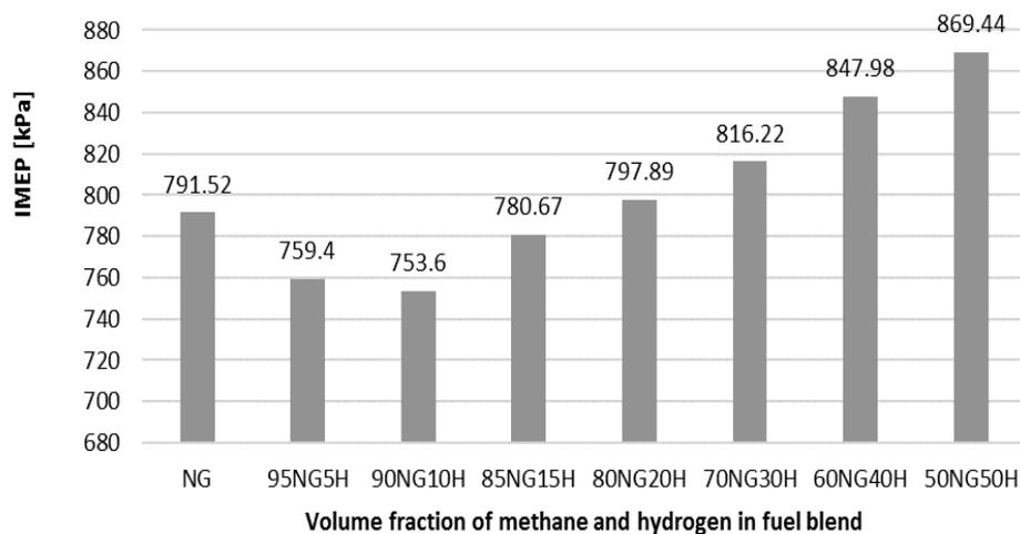
Fig. 5. IMEP for the engine fueled by methane enriched with hydrogen, at 2500 rpm; WOT and  $\lambda = 1.0$
