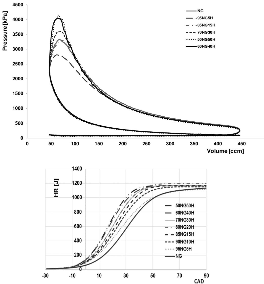
Fig. 4. p-V diagram and heat-release function for the engine fueled by methane, enriched with hydrogen, at 2500 rpm; WOT and  $\lambda = 1.0$
