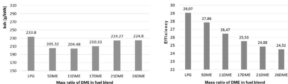
Fig. 10. Brake specific fuel consumption and Engine efficiency for all LPG DME blend
