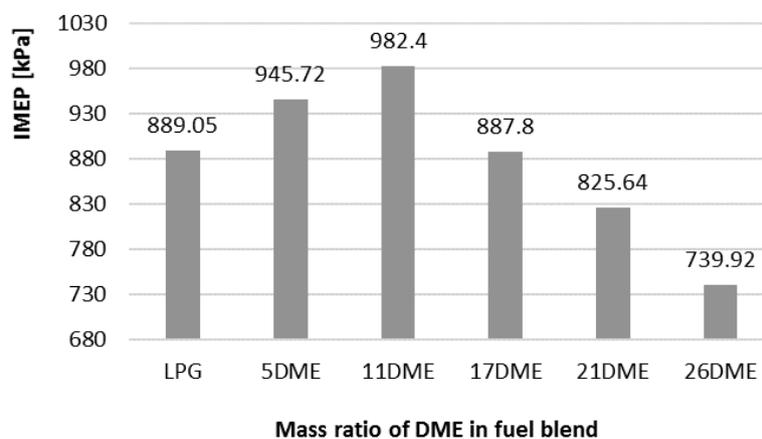
Fig. 7. IMEP for the engine fueled by LPG–DME mixtures, at 2500 rpm; WOT and  $\lambda = 1.0$
