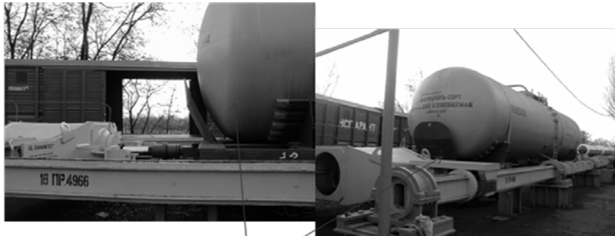
the tank-wagon in the stand for tensile and compression
