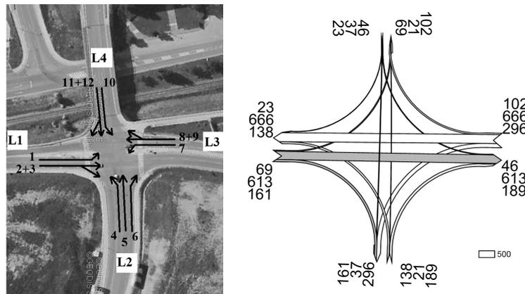
Fig. 3. Junction legs (L1-4) and traffic flows labelling according to TP 10/2010 rules (on left), traffic state during traffic peak (on right)
