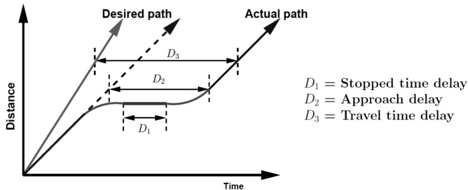
Fig. 1. Illustration of delay measures [9]
