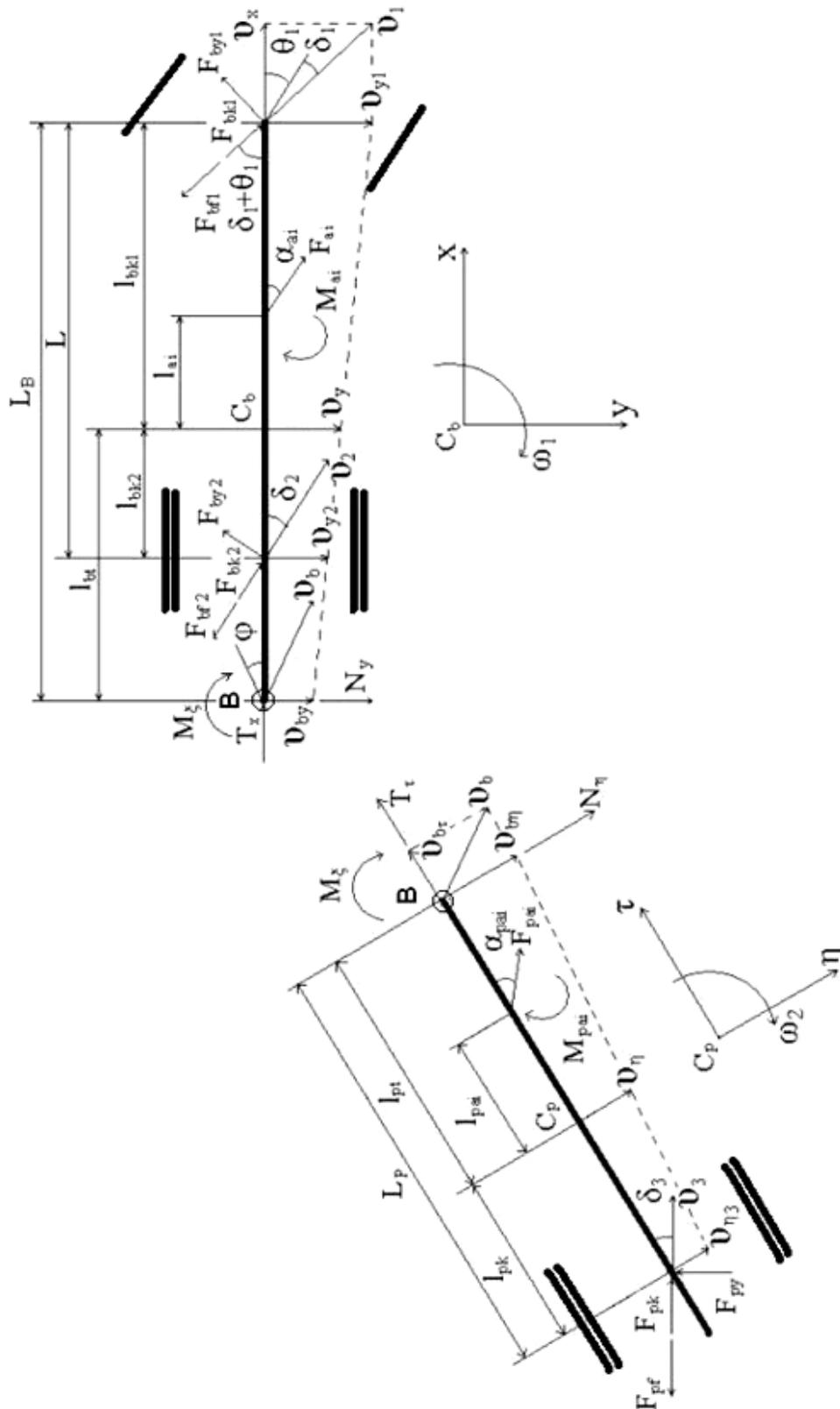
Fig. 1. Mechanic-mathematical model of an articulated vehicle
