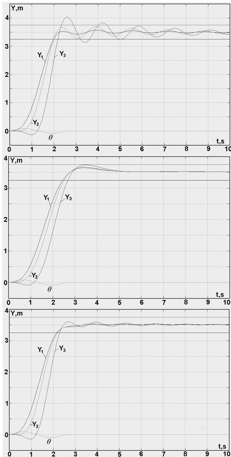
Fig. 3. Trajectories of the vehicle axles: a – no additional resistance; b – with viscous resistance; c – with dry friction resistance;  $Y_1, Y_2, Y_3$  – lateral displacement of the center of respective vehicle axles
