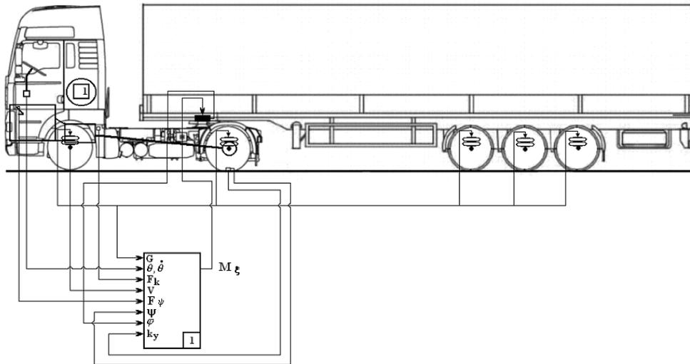
Fig. 4. A block scheme of a system for active control of the resistant moment
