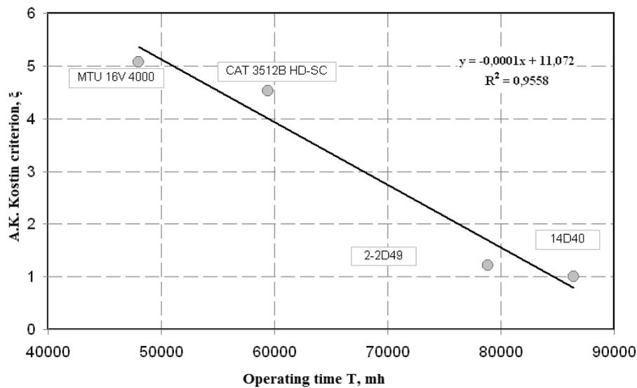
Fig. 1. Inter-reliance of operating time (T) of AB “LG” cargo locomotives and indirect criterion ζ
