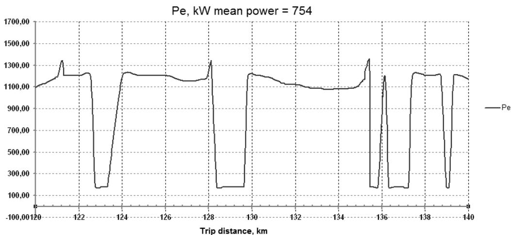
Fig. 6. 2M62M locomotive load cycle parameters on track Vaidotai-Kybartai (traction restriction coefficient 0.83)
