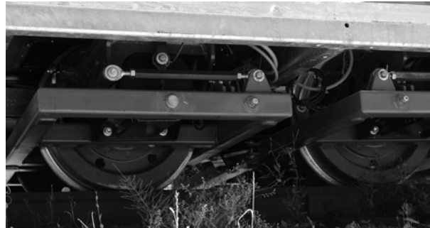
Fig. 4. The rotary bogie with independent rotating driven wheels
