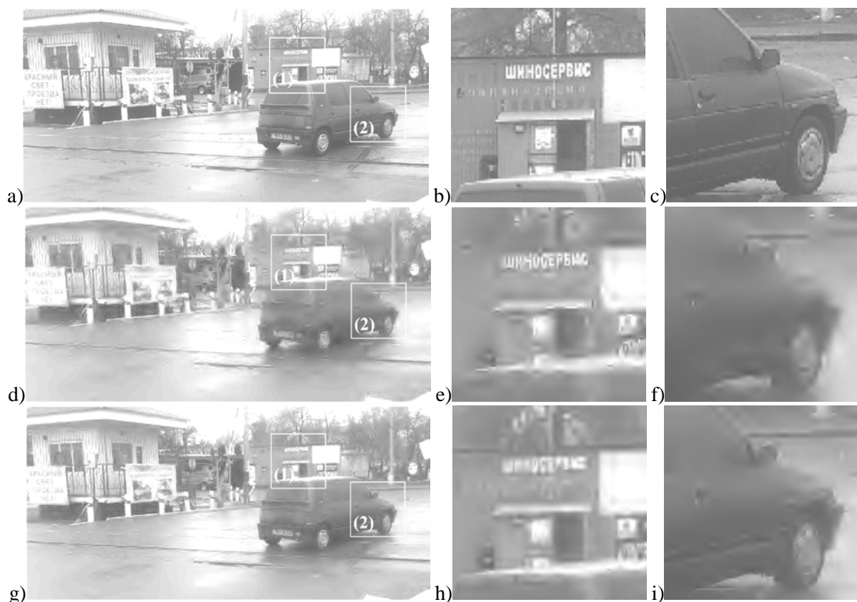
Fig. 3. Compared images: (a)–(c) – original, (d)–(f) – plain SPIHT compressed, (g)–(i) – proposed pre-processing with SPIHT
