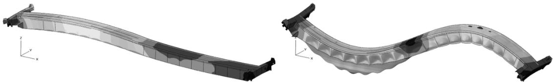
Fig. 11. IX<sup>th</sup> form of vibration frequency 20,77 [Hz], X<sup>th</sup> form of vibration frequency 23,95 [Hz]
