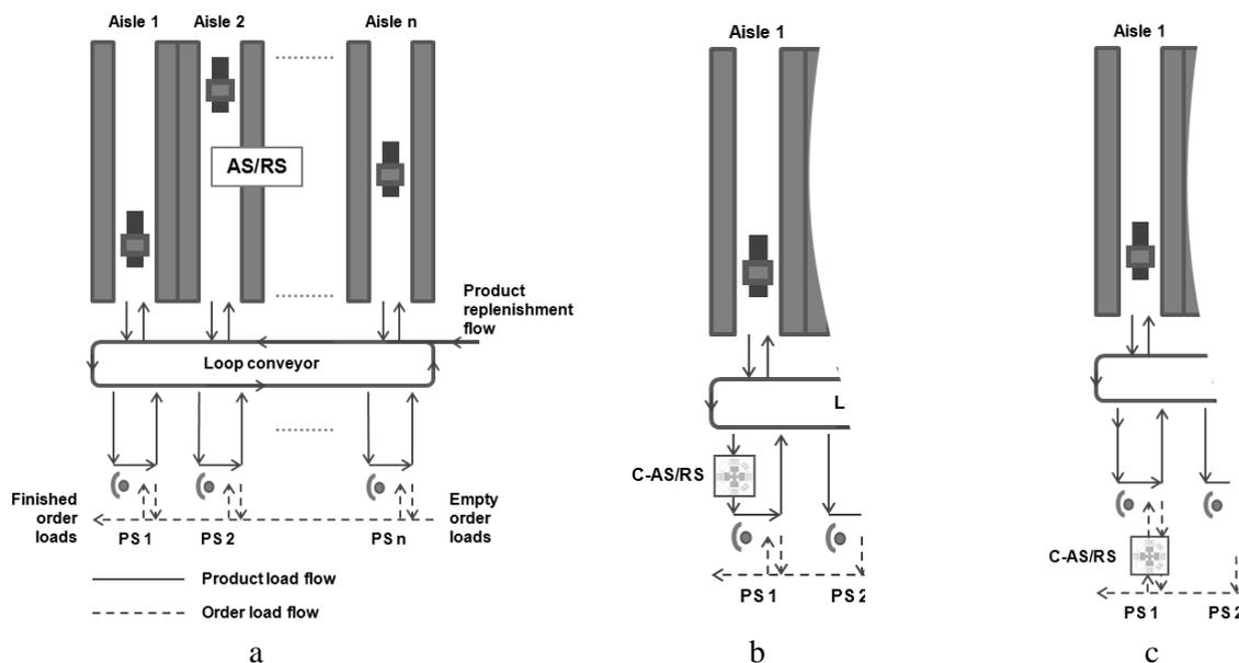
Fig. 1. a) End-of-aisle OPS; C-AS/RS integration into end-of-aisle OPS, b) option 1, c) option 2
