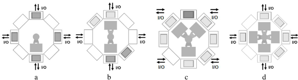
Fig. 3. C-AS/RS configurations with 4 I/O positions: a) 1 LHD; b) 2 LHD; c) 3 LHD; d) 4 LHD
