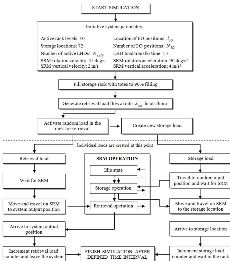
Fig. 4. C-AS/RS simulation model
