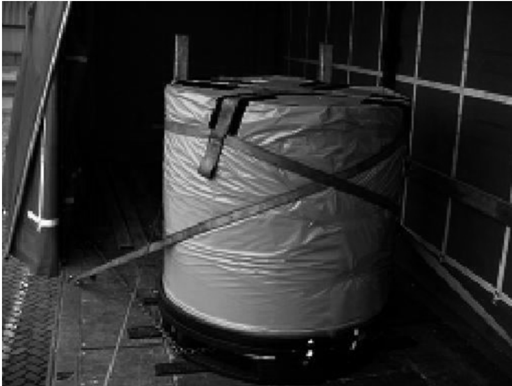
Fig. 5. Protection of steel coils carried with bore vertically
