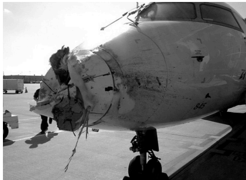
Fig. 1. Aircraft damage caused by bird strike (Source: photoblog.nbcnews.com)
