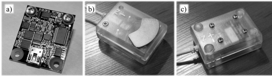
Fig. 4. a) PHIDGET 1056 measuring circuit, b, c) measuring head with magnetic holder
