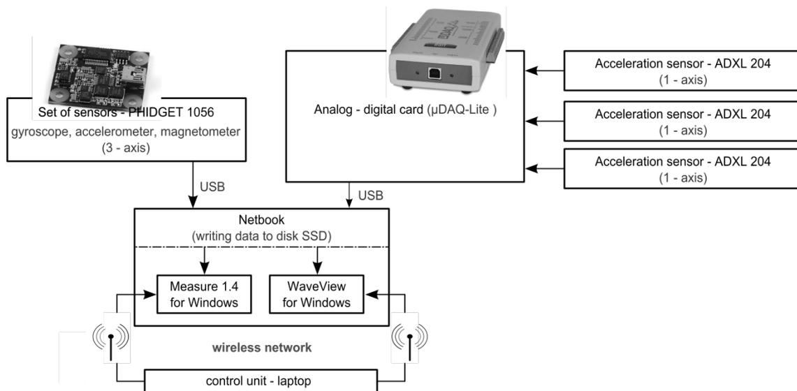
Fig. 3. Block diagram of the two independent measurement channels
