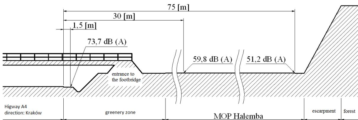
Fig. 5. Soil profile of the terrain MOP Halemba
