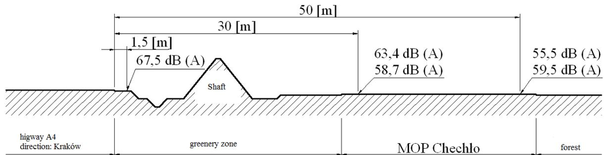
Fig. 2. Soil profile of the terrain MOP Chechło
