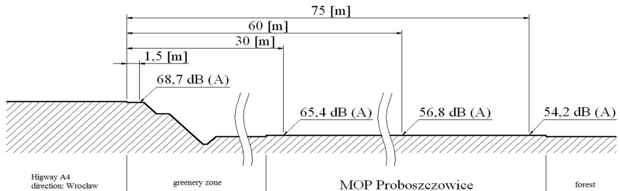
Fig. 3. Soil profile of the terrain MOP Proboszczowice
