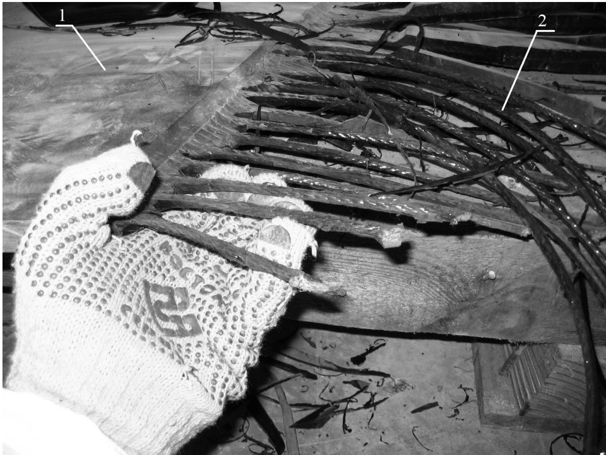
Fig. 1. General view of conveyer belt failure on Joint-Stock Company "Altyntau Kokshetau": 1 - conveyer belt; 2 – rope
