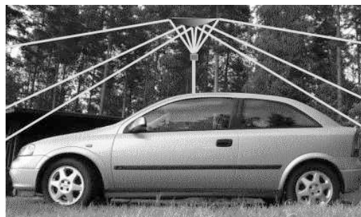
Fig. 4. An omni-directional camera arrangement for traffic safety measurements
