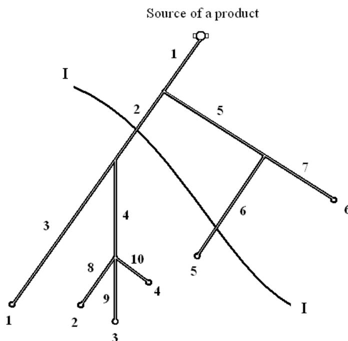
Fig. 1. The scheme of pipeline and the position of soil displacement line I-I
