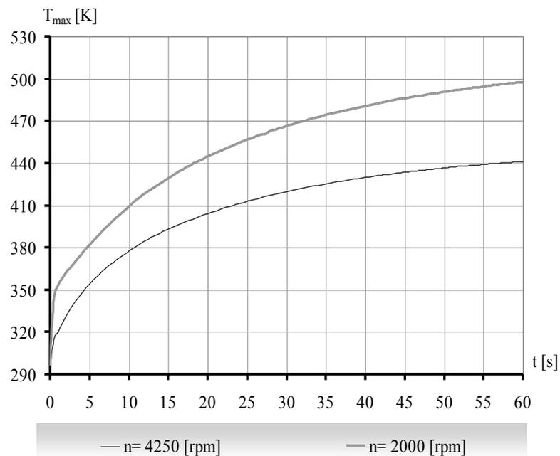
Fig. 6. The diagrams of maximum temperature on the surface of the piston head
