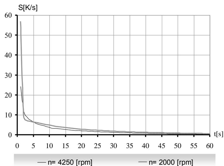
Fig. 7. The course of the speed of the temperature changes on the surface of the piston engine
