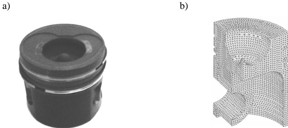
Fig. 3. The piston engine: a) real element , b) discrete model
