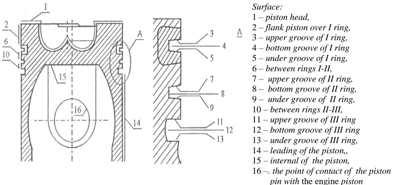
Fig. 4. Surface exchange heat of the piston
