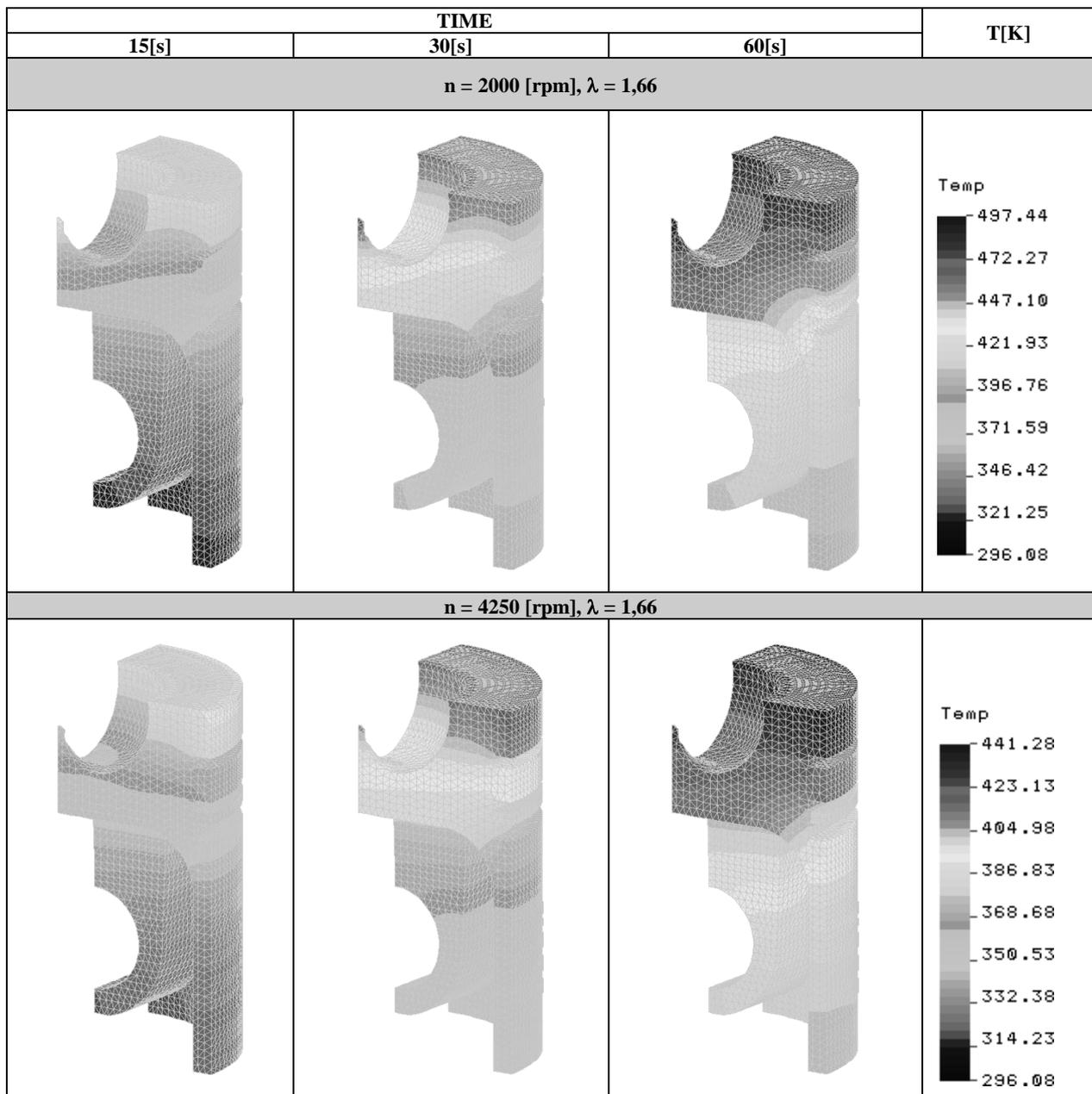
Fig. 5. The following phases warming up of the piston engine
