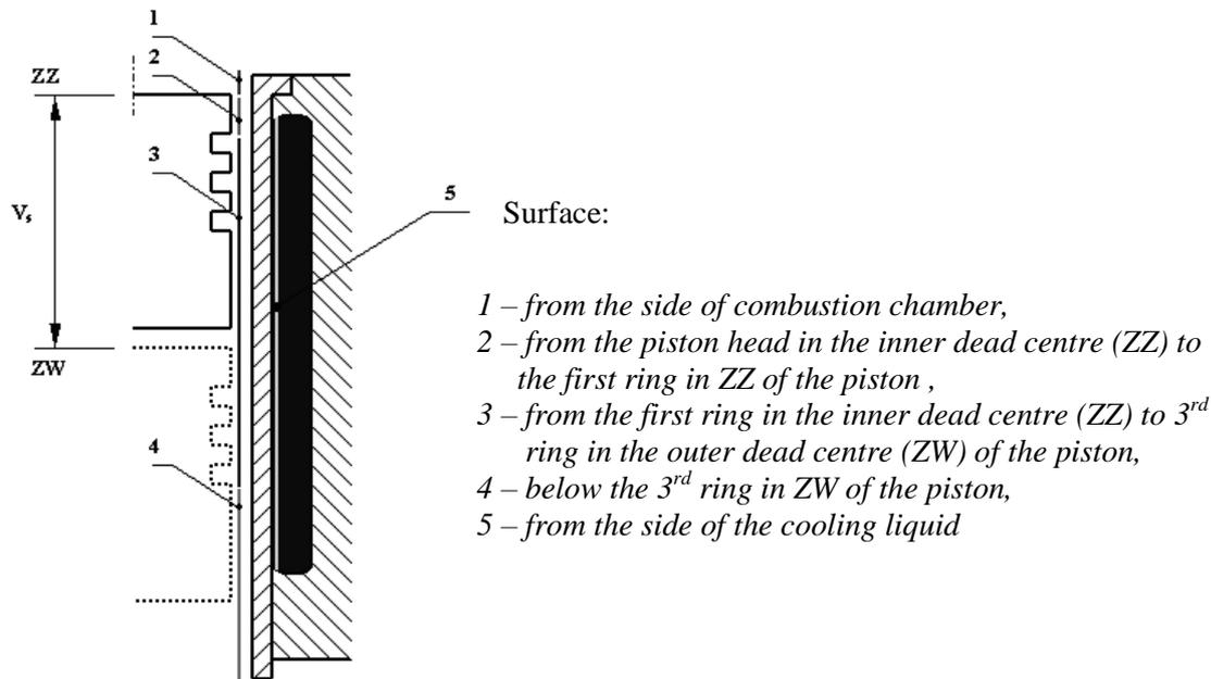
Fig. 1. The wet cylinder sleeve
