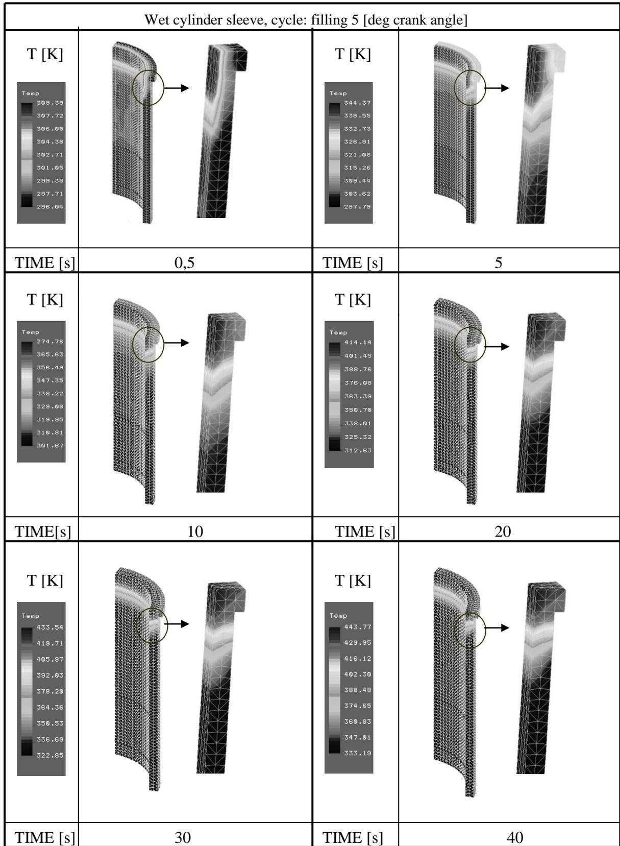
Fig. 2. Distribution of temperature in the wet cylinder sleeve
