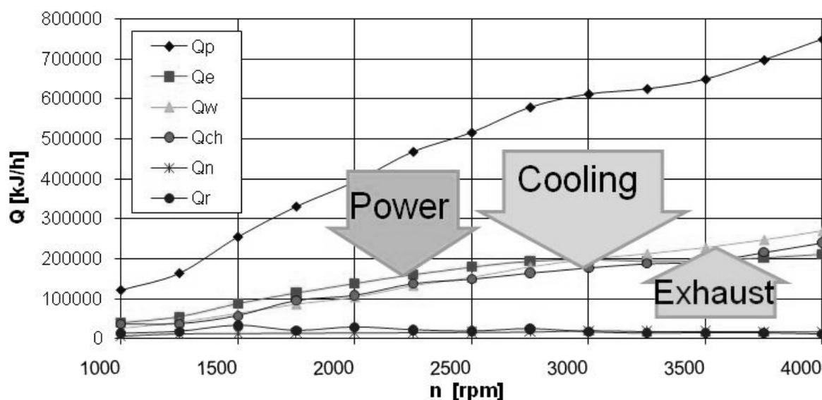
Fig. 1. Comparison of heat engine 4CT90 streams (designation:  $Q_p$  – heat from the combustion of fuel spilled,  $Q_e$  – heat converted into useful work,  $Q_{ch}$  – dissipate heat to the cooling system,  $Q_w$  – convection heat from the exhaust gases,  $Q_r$  – the rest of the balance, and the heat discharged into the environment from the hot walls of the engine and other losses)
