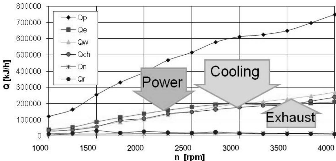
Fig. 1. Comparison of heat engine 4CT90 streams (designation:  $Q_p$  – heat from the combustion of fuel spilled,  $Q_e$  – heat converted into useful work,  $Q_{ch}$  – dissipate heat to the cooling system,  $Q_w$  – convection heat from the exhaust gases,  $Q_r$  – the rest of the balance, and the heat discharged into the environment from the hot walls of the engine and other losses)
