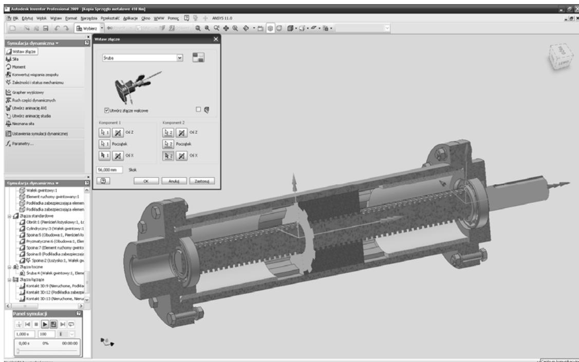
Fig. 3. Estimation of the „screw thread” bound type between sliding sleeve and coupling shaft
