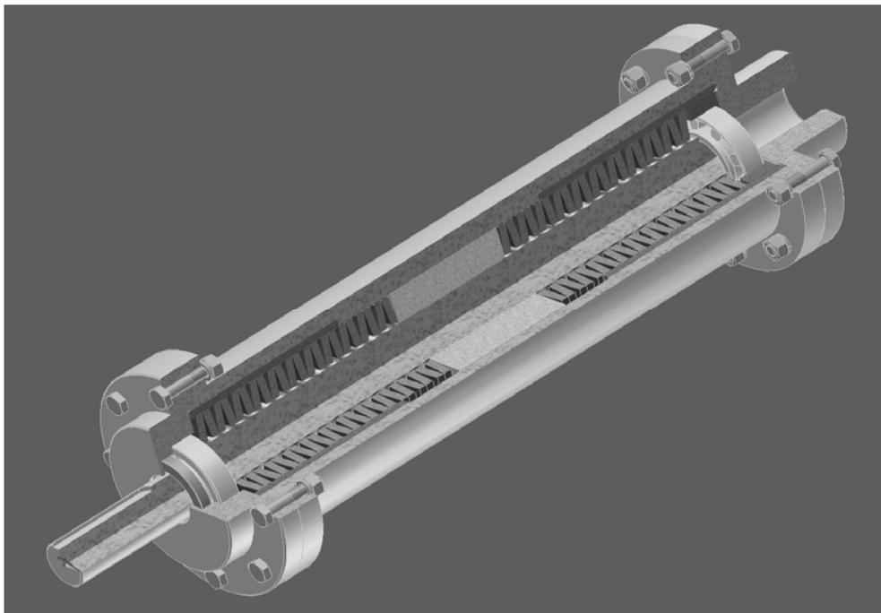
Fig. 2. View of the two-way prototype of the metal flexible torsional coupling
