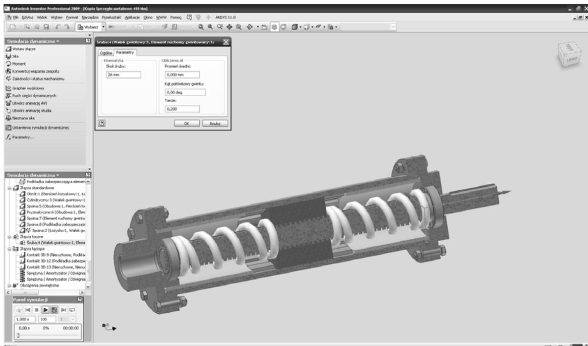
Fig. 5. Example estimation of friction factors between sliding sleeve and coupling shaft
