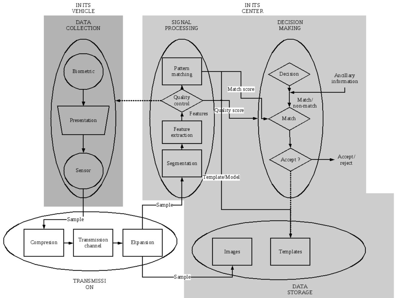
Fig. 2. Modified generalised biometric system model
