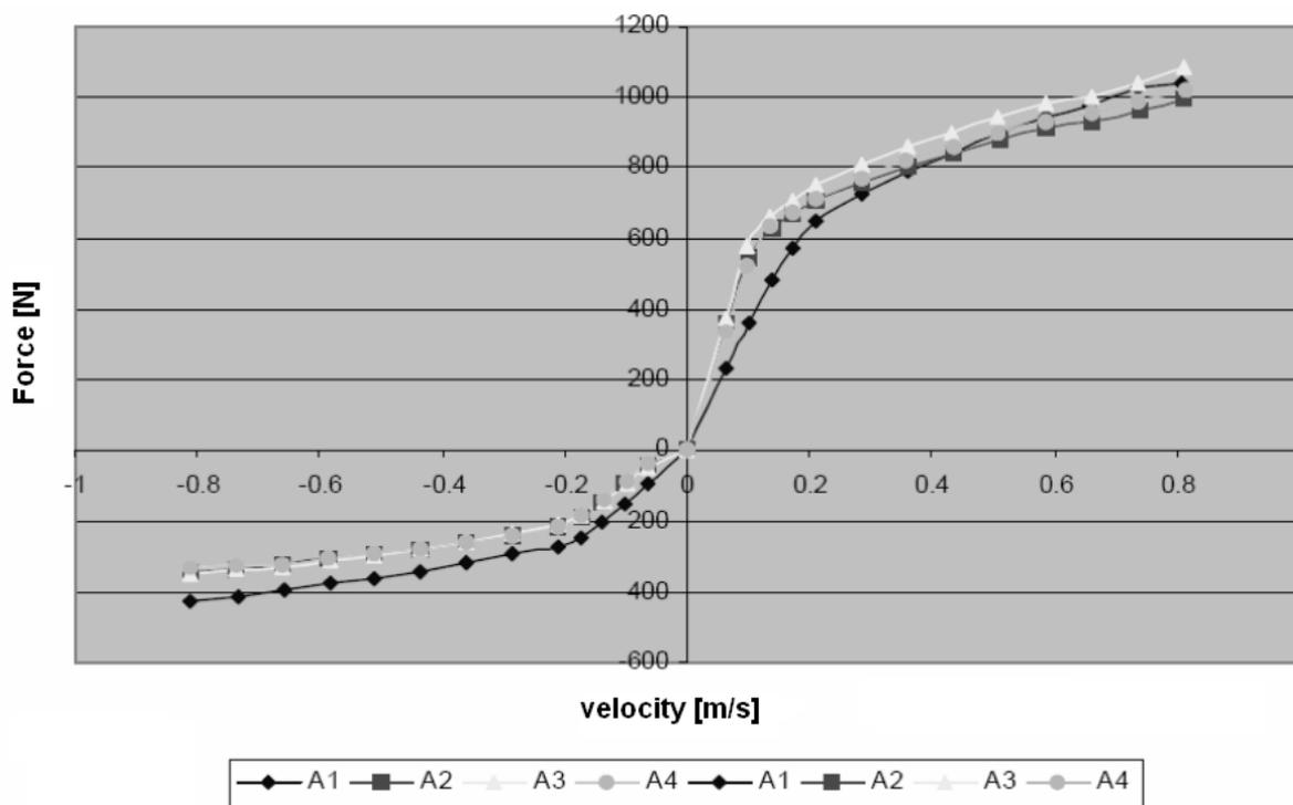
Fig. 2. Dumping characteristic of new shock absorbers
