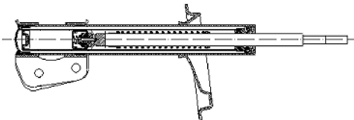
Fig. 3. Shock absorber construction
