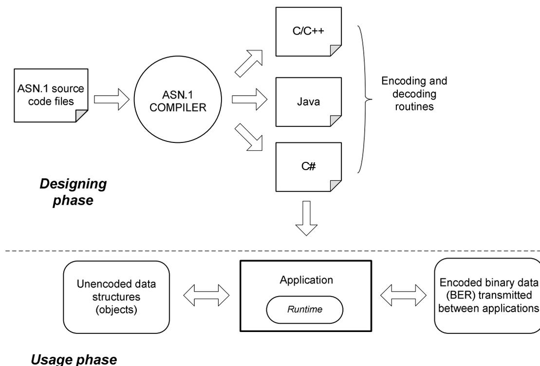
Fig. 1. Designing and usage of communication software in ASN.1
