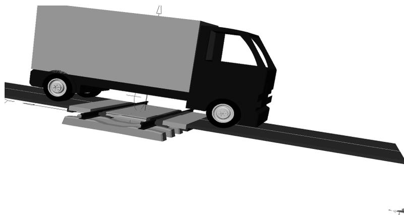
Fig. 4. Simulation of a truck passing over the railway crossing in the MSC VisualNastran 4D system
