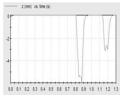
Fig. 10. Amplitude of displacements of slab1 with tension force of 60 kN and the truck speed - 50 km/h
