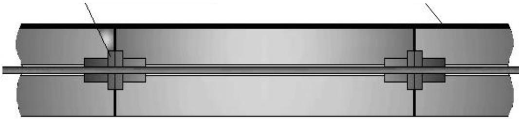
Fig. 5. Conception of driving the strings through concrete slabs – longitudinal section through a slab
