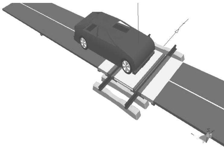
Fig. 3. Simulation of a car driving over the railway crossing in the MSC VisualNastran 4D system
