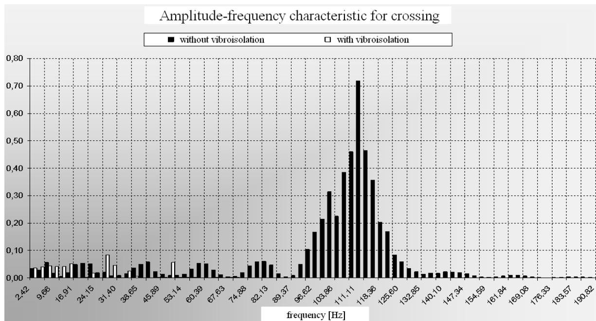
Fig. 12. Amplitude - frequency characteristic for crossing with the application of vibroisolation and without it
