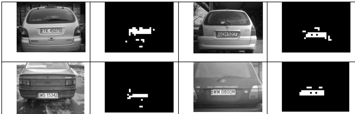
Fig. 8. The results of the license plate localization algorithm
