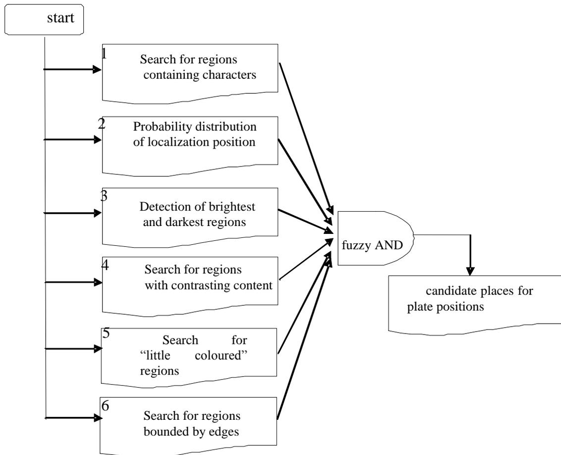
Fig. 1. Diagram of the license plate localization algorithm
