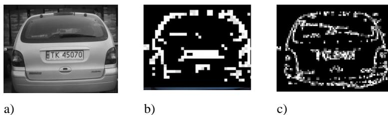
Fig. 2. a) Original image, b) FFT based detection, c) Density of vertical edges
