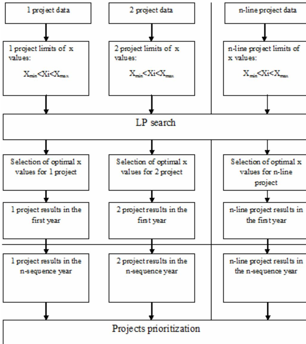
Fig. 10. Block scheme of the efficiency evaluation model
