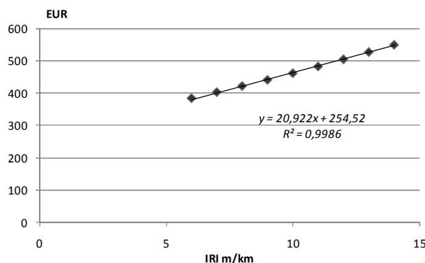
Fig. 2. VOC correlation between the surface roughness in case of the gravel road
