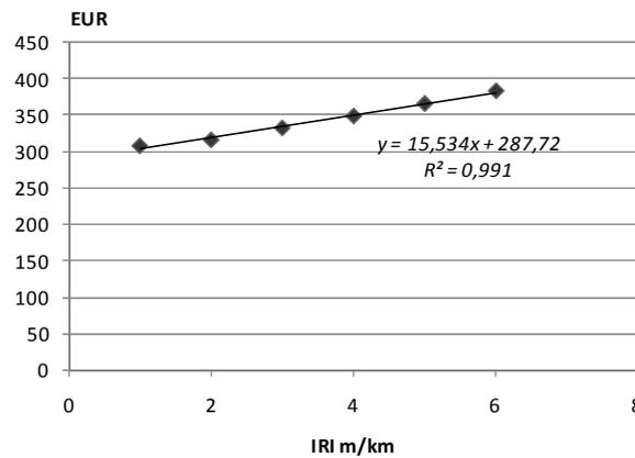
Fig. 1. VOC correlation between the surface roughness in case of the paved road
